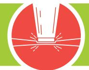
Make sure that cords are not pinched in doors, windows or under heavy furniture, which could damage the cord's insulation.
