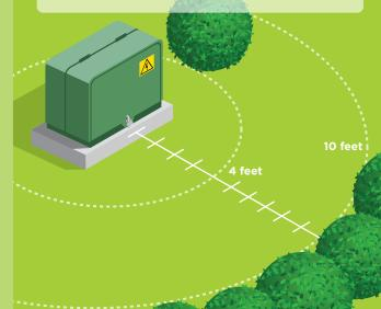
Never dig near a pad-mounted transformer. They are surrounded by underground cables. Hitting the cable could result in electrical shock or disruption of service.
